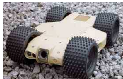
QinetiQ North America’s Technology Solutions Group has launched its new Dragon Runner Small Unmanned Ground Vehicle (SUGV). Dragon Runner SUGV is the first fully modular ground robot system
