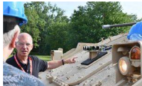
A U.S. Army TARDEC engineer explains the operation of the forward-facing camera package that enables depth perception during closed-hatch driving. TARDEC, with Honeywell Aerospace and DARPA, are demonstrating a proof-of-concept for closed-hatch driving using high-resolution stereo vision at Detroit Arsenal in Warren, Michigan, June 12, 2018.
