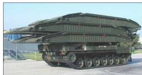
Munich/Koblenz -- The Federal Office of Bundeswehr Equipment (BAAINBw) and Krauss-Maffei Wegmann (KMW) have signed an agreement on the procurement of seven Leguan bridge laying systems on the Leopard 2 chassis in
